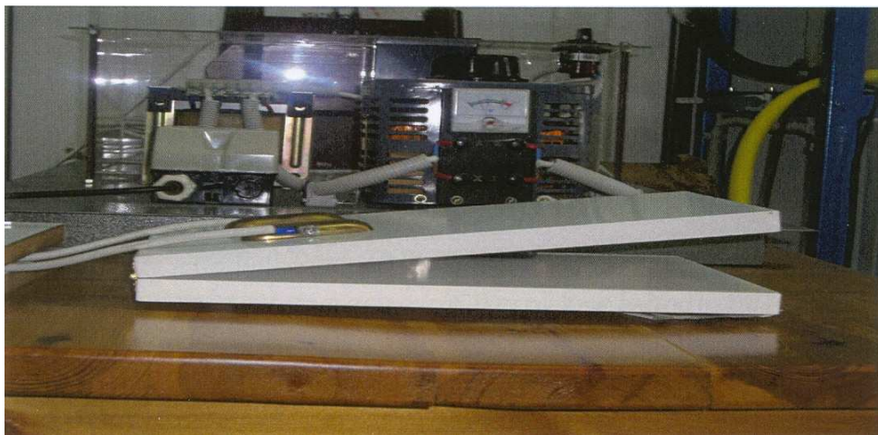
Fig. 3: The inclined Plane test setup (side view)
