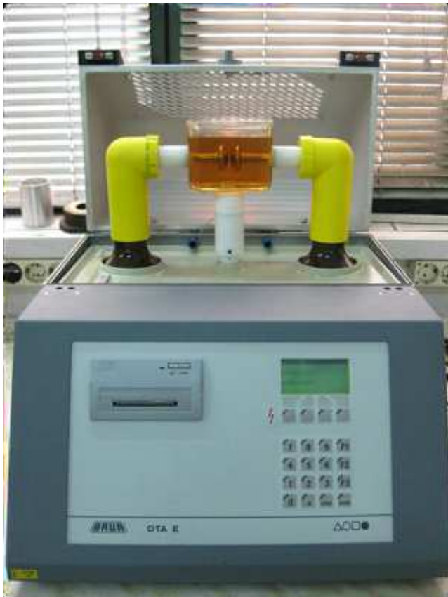
Fig. 1: Device for the measurement of dielectric strength
