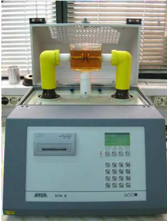
Fig. 1: The test cell for breakdown voltage measurements
