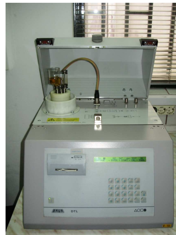
Fig.2: Device for measurement of \tan\delta and resistivity
