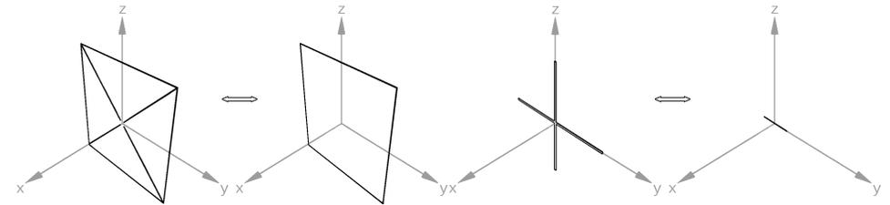
Fig. 12: Almost equivalent antennas in terms of radiation
