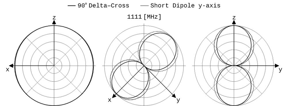
Fig. 14: 90° Delta-Cross and Short dipole on y-axis radiation
