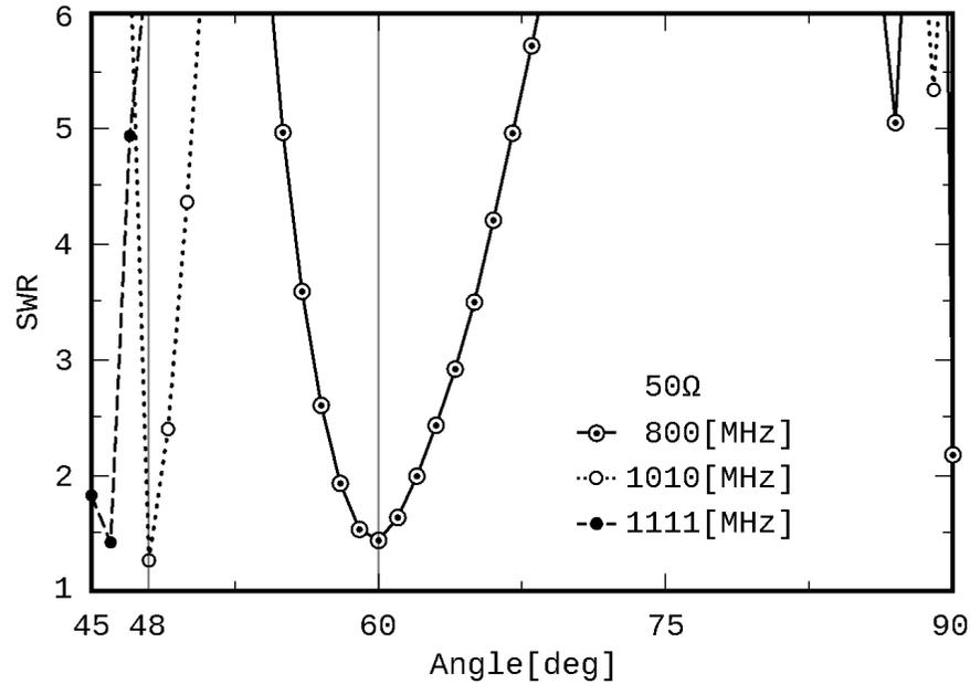
Fig. 16: SWR for 50 [Ω] characteristic impedance
