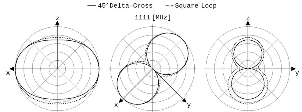
Fig. 13: 45° Delta-Cross and Square loop radiation
