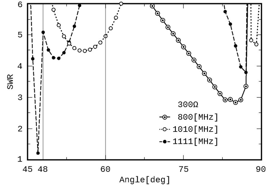
Fig. 18: SWR for 300 [Ω] characteristic impedance
