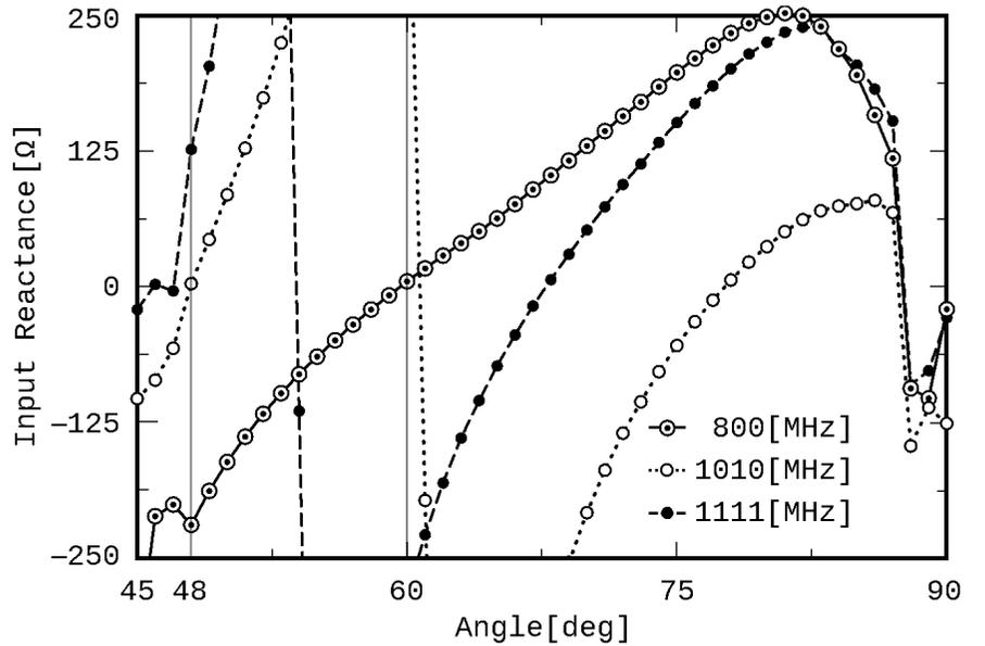
Fig 19: Input Impedance versus base angle
