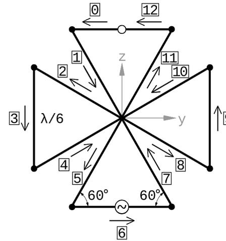
Fig. 1: The Planar Delta-Cross Shaped Loop antenna
